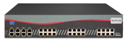
or E1 R2 ports in a single, 19" 2U chassis. Additional PSTN/analog phone ports can be provided by connecting external <u>Astribank</u> units via the USB2 ports, for a total of up to 672 PSTN/analog phones ports, up to 1000 users and up to 300 concurrent calls.
