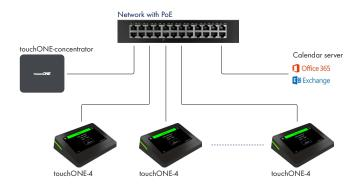
The touchONE-4 connects to a local data network equipped with PoE infrastructure. All workplace interfaces communicate with the touchONE-concentrator, which provides system setup and communication with calendar servers. One interface is used for each workplace and one data concentrator is required for every 100 workplace interfaces. The data concentrator must be connected to the same local network as all touchONE-4 workplace interfaces.
